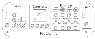
$HIGHPASS\ FILTER ^*-GATE-COMPRESSOR-EQUALIZER-LIMITER ^*$
