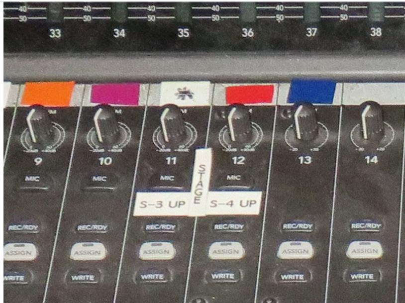
Channels 11 & 12 also receive line inputs from the S-3 and S-4 inputs on the stage.
