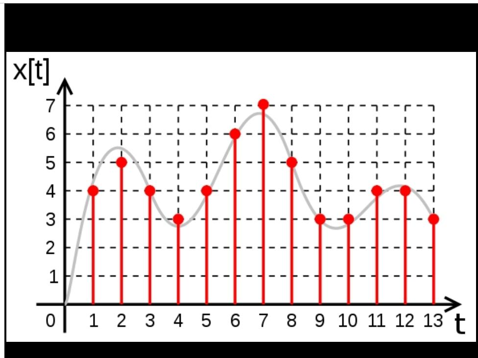
The big difference between analog and digital waves is Digital signals must have a finite set of possible values. Where as Analog waves are smooth and continuous, digital waves are stepping, square, and discrete
