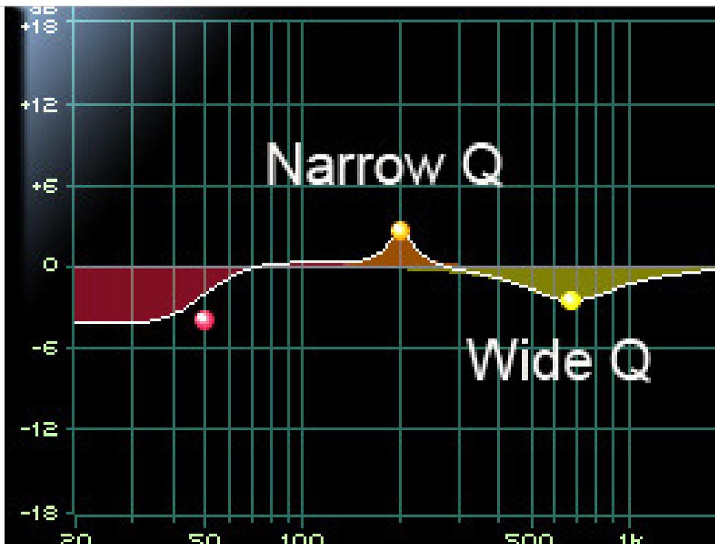
This graph shows a Parametric EQ in use. In the middle, we see an orange dot on the 200Hz line and it's gain has been increased 3dB. It has a narrow "Q" of about 100Hz.
