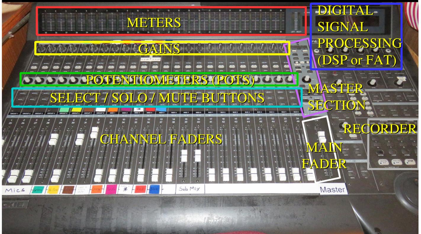
**METERS:** Display the signal input levels
