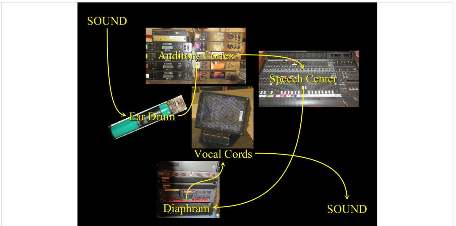
The sound enters the Microphone, vibrating a diaphragm that converts the vibrations into a radio frequency. The frequency is picked up by the Receivers and converted into Mic Level electronic signals.
