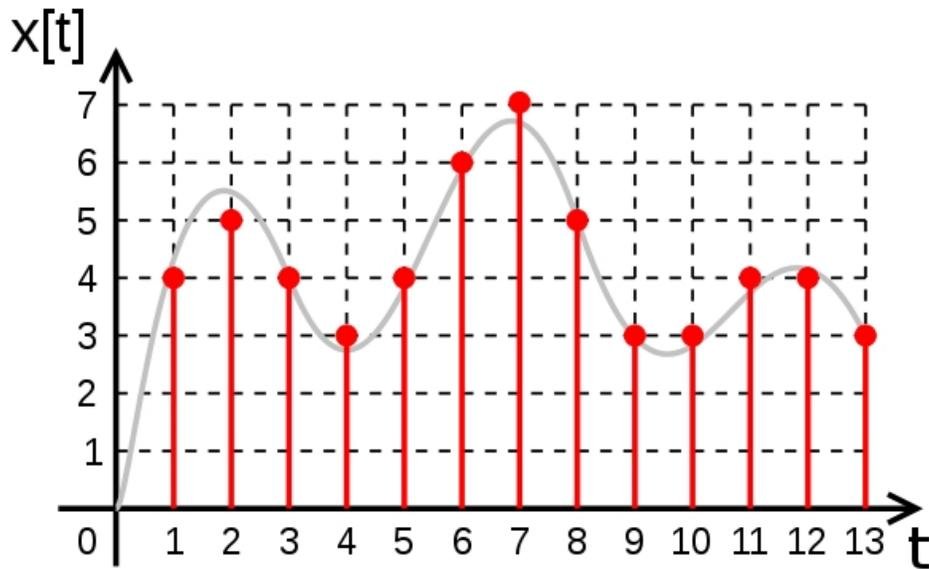
The big difference between analog and digital waves is Digital signals must have a finite set of possible values. Where as Analog waves are smooth and continuous, digital waves are stepping, square, and discrete
