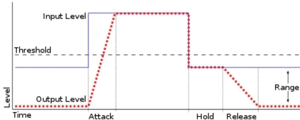
This graph shows the blue input level is lower than the threshold, so the gate stays closed, not allowing the output to pass. When the input passes the threshold, the gate opens (attack). When the signal drops below the threshold, the gate closes (release). This mixer has no “hold” setting.
