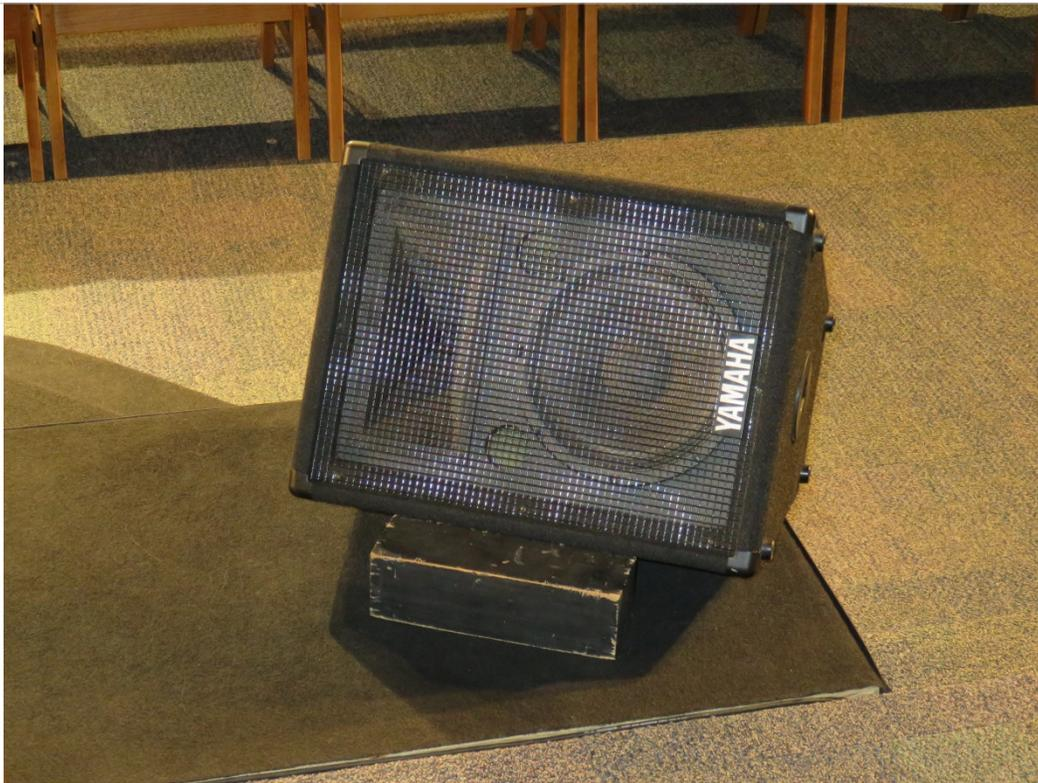
And to the floor wedges or Monitor Speakers. Speaking of which, we don't have true monitor Speakers. True monitor speakers have a cone of Sound you must stand in to hear the speaker, thus preventing other mics from picking up the speaker.
