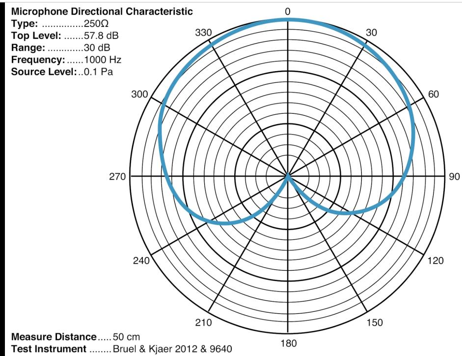
This graph shows the pickup angles. 0 at the top picks up the most sound. Turning the mic away so it's  $90^\circ$  from the source picks up  $\sim 2/3$  of the sound. Having the mics butt pointed toward a speaker means it won't pickup any sound from that source.
