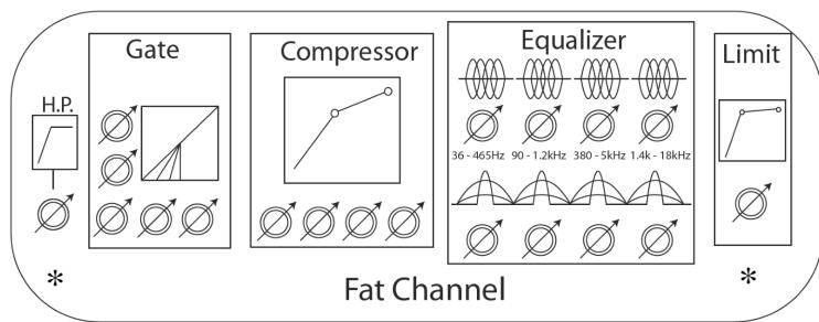
HIGHPASS FILTER\* – GATE – COMPRESSOR – EQUALIZER – LIMITER\*
