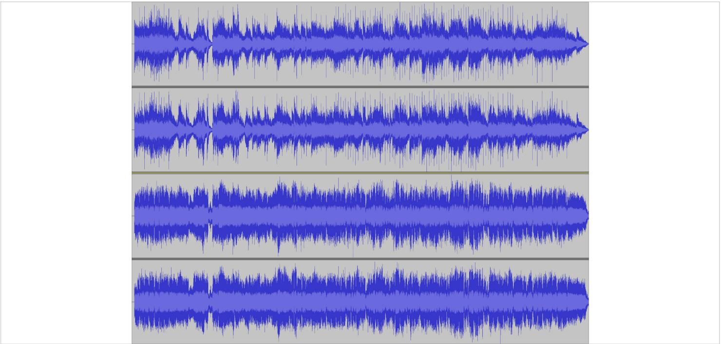
This image shows two wave forms. The two tracks on top have no compression. Showing the wide range of Dynamics. The Dynamic range is just the difference between the loudest and quietist parts.
