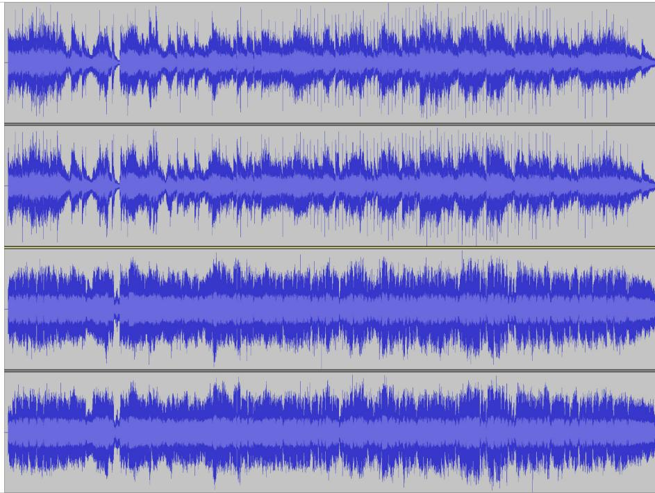
This image shows two wave forms. The two tracks on top have no compression. Showing the wide range of Dynamics. The Dynamic range is just the difference between the loudest and quietest parts.
