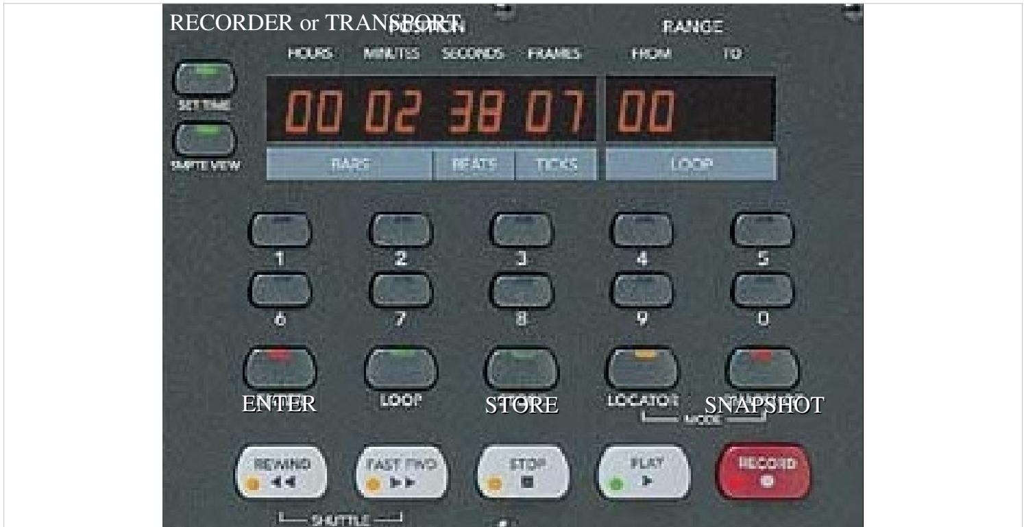
This area allows us to store our mixer settings in “Snapshots”. We can make a file on the computer that stores 99 snapshots. To store a Snapshot, press the Snapshot button then type in the Snapshot# from 01 to 99. Then press Store and then Enter. This only stores the Snapshot to the file. The file must then be saved by pressing CTRL+S on the keyboard.
