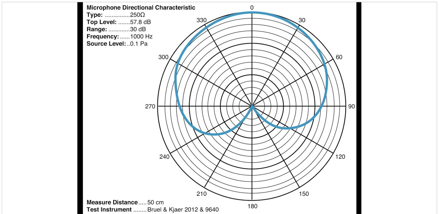
This graph shows the pickup angles. 0 at the top picks up the most sound. Turning the mic away so it's 90° from the source picks up ~2/3 of the sound. Having the mics butt pointed toward a speaker means it won't pickup any sound from that source.
