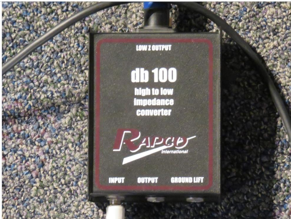
If someone brings an electro-acoustic guitar, they will need a Direct Input (DI) BOX to plug their guitar into using a 1/4" audio plug. The DI BOX then uses an XLR cable to connect to the Organ Mixer or the stage connections. We'll cover cables and plugs a little later.
