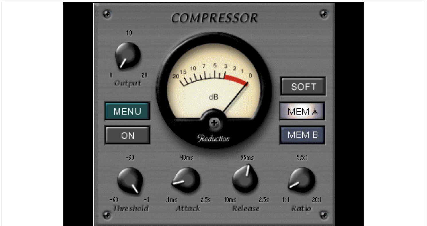
Considering the Gate prevents weak signals from passing into the channel, the Compressor reduces strong signals.
