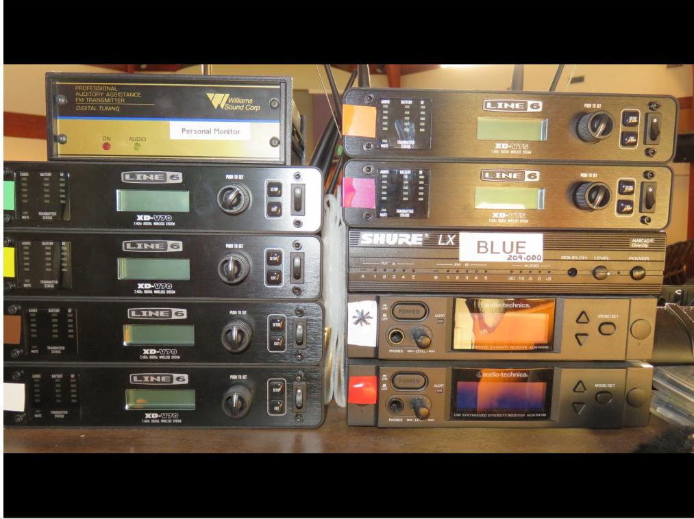
The mics and packs send their RF signals to these receivers which send the signal to the splitters
