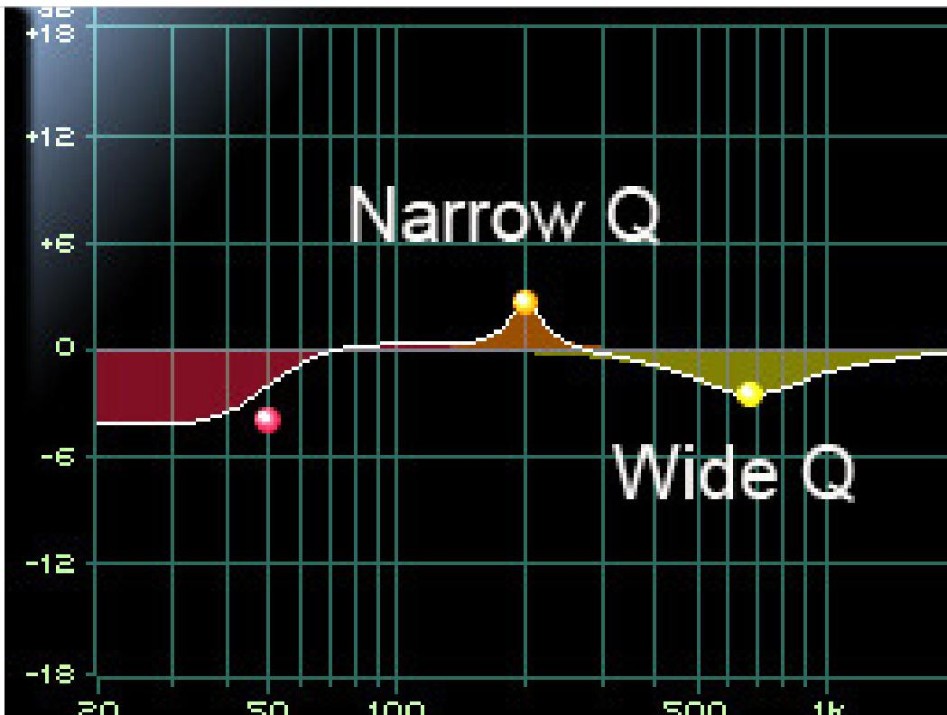
This graph shows a Parametric EQ in use. In the middle, we see an orange dot on the 200Hz line and it's gain has been increased 3dB. It has a narrow "Q" of about 100Hz.
