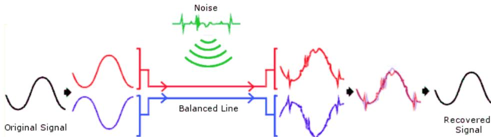
A Balanced cable has three wires. Two signal wires to carry the signal data and a third ground wire. The two signal wires, carry the same signal, except the signal on one of the wires has a reversed polarity. So one is opposite of the other. If any noise is picked up by the wires the noise will be identical on both signal wires.
