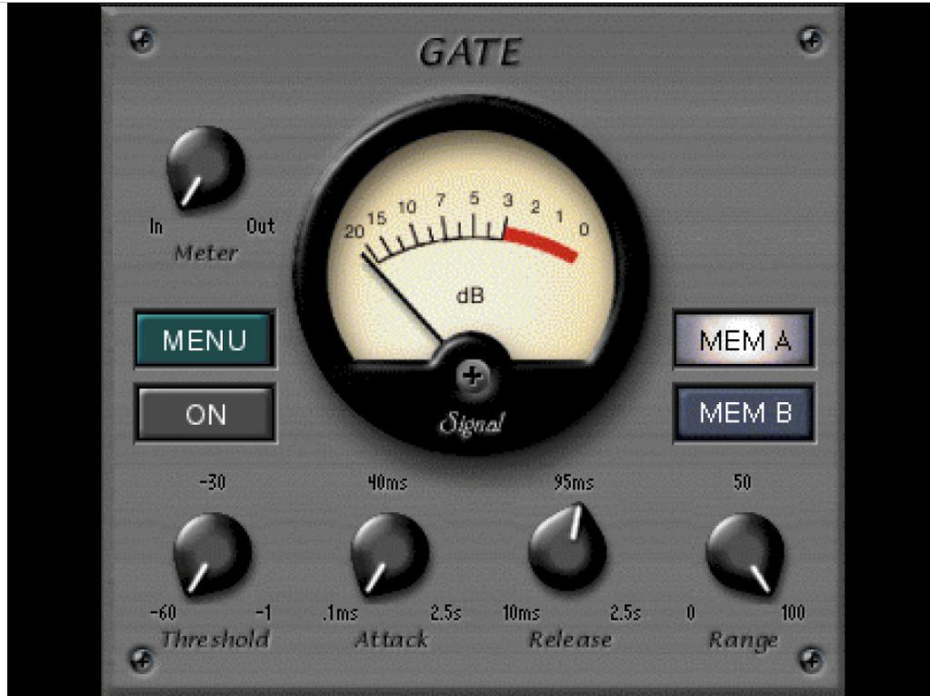
The Gate, allows or prevents signals from passing through the channel.
