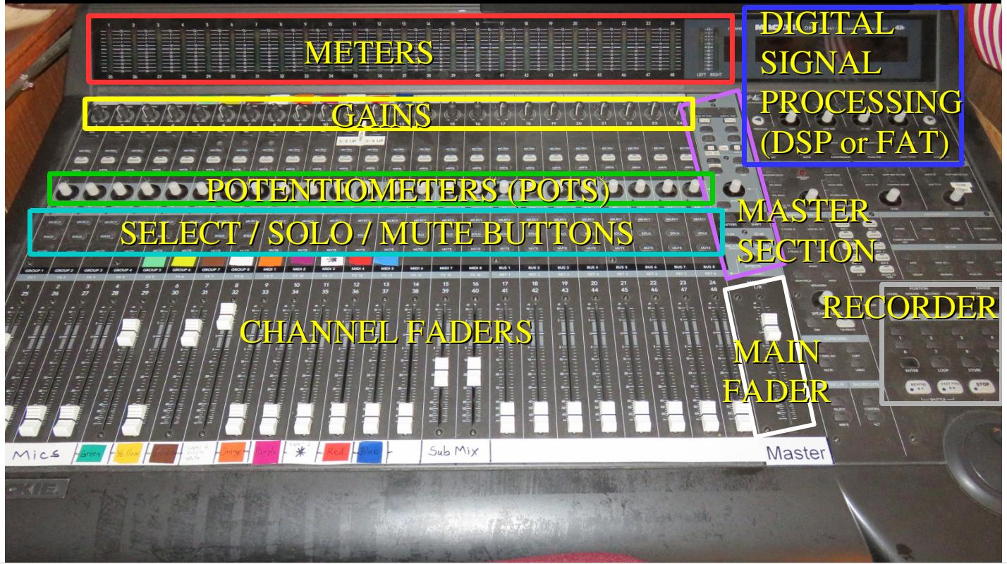
**METERS:** Display the signal input levels
