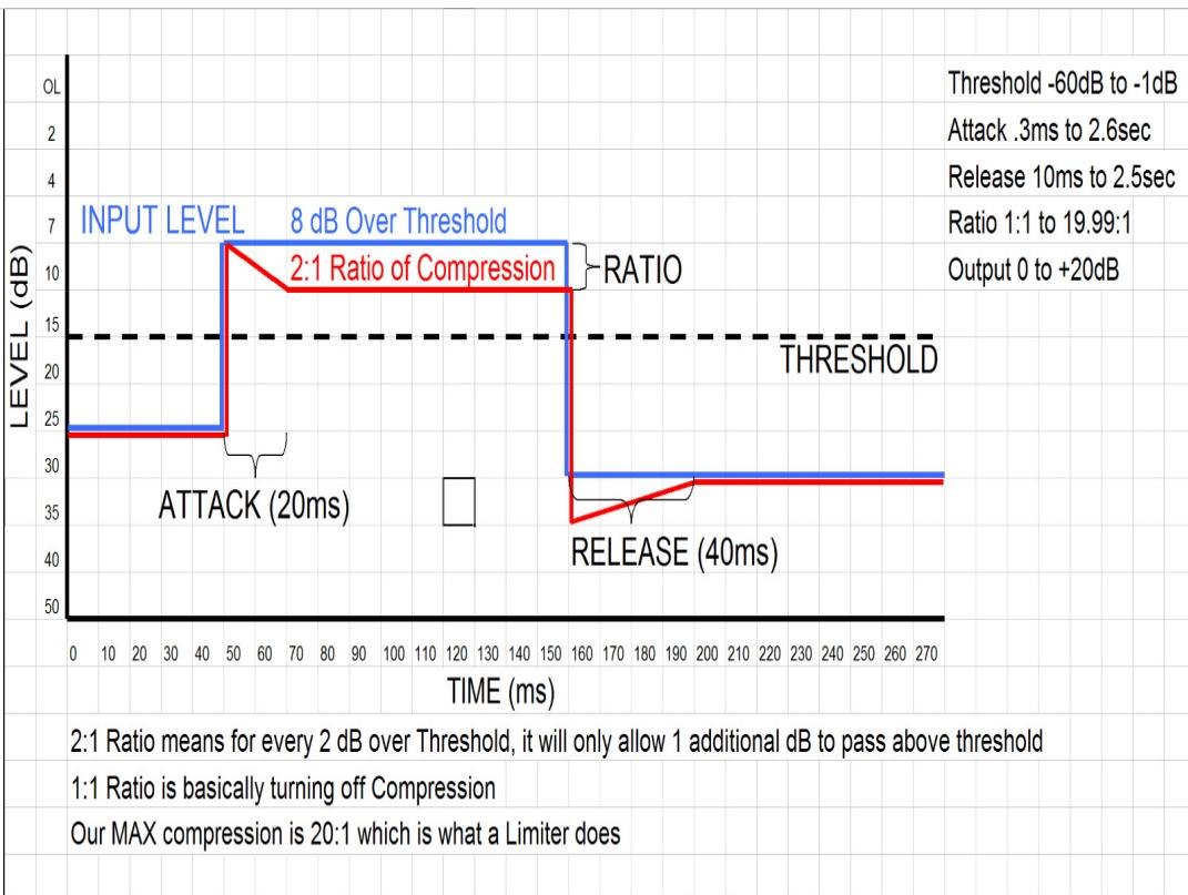
We can see in this graph, as long as the blue input level is below the threshold, the compressor will not affect the output level. When the input does exceed the threshold, the compressor takes 20ms to activate, or reduce the output level by the ratio of 2:1. The compressor will allow 1dB of signal to exceed the threshold and pass through the channel, for every 2dB that's over the threshold. When the input drops below the threshold, the compressor will take 40ms to match the input level.
