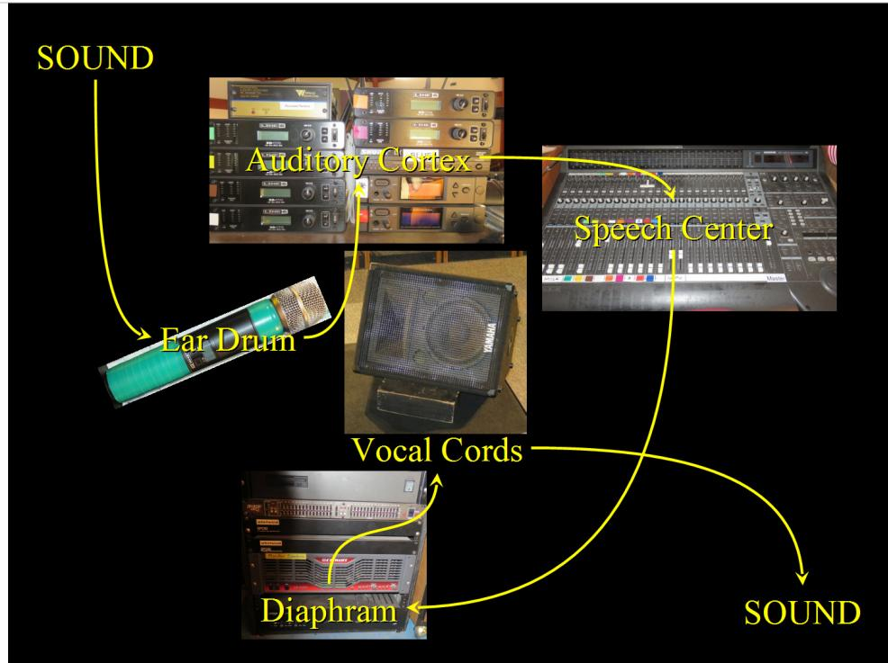
The sound enters the Microphone, vibrating a diaphragm that converts the vibrations into a radio frequency. The frequency is picked up by the Receivers and converted into Mic Level electronic signals.
