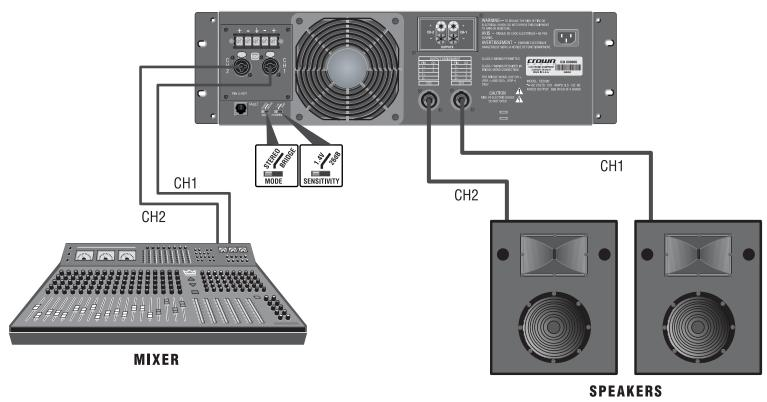
Figure 2.9 Typical System Wiring, Stereo Mode
