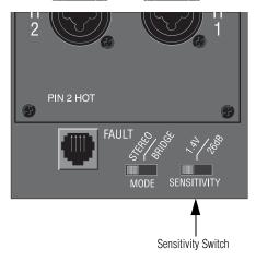
Figure 2.12 Location of Input Sensitivity Switch
