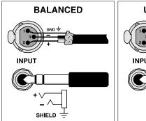
Figure 2.3 Balanced Input Connector Wiring
