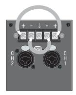
Figure 2.10 Jumper Placement to Parallel the Inputs
