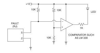
Figure 4.3 Fault Status LED Circuitry
