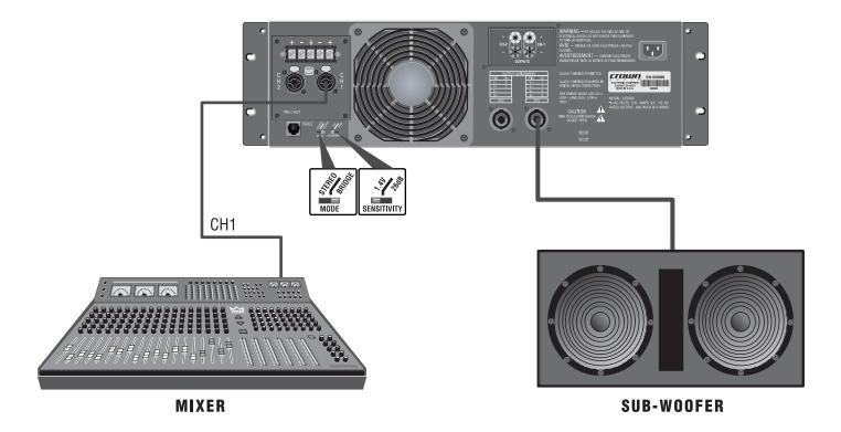
Figure 2.11 Typical System Wiring, Bridge-Mono Mode
