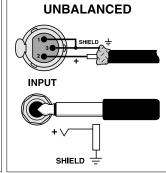
Figure 2.4 Unbalanced Input Connector Wiring
