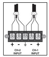
Figure 2.5 Barrier Strip Input Wiring: Balanced Signal In
